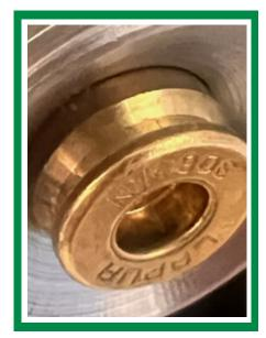
The root cause of the incident appears to have been due to a fault in the initial barrel chambering. The rifle owner is in discussion with the supplier of the barrel regarding a remedy.
